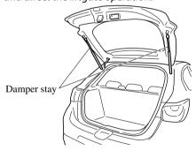
Do not modify or replace the liftgate damper stay. Consult an expert repairer (we recommend an Authorised Mazda Repairer) if a liftgate damper stay is deformed or damaged for reasons such as a collision or if there is some other problem.
