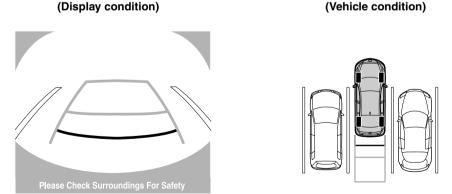
6. When the shift lever/selector lever is shifted from R to another shift lever/selector lever position, the screen returns to the previous display.
