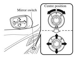
After adjusting the mirror, lock the control by rotating the switch to the centre position.
