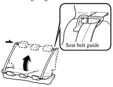
2. Press the seatback rearward and lock it in place. After returning the seatback to its upright position, make sure it is securely locked.
