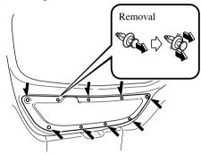
3. Using a flathead screwdriver, open the inner cover.
