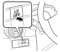
The Lane-keep Assist System (LAS) & Lane Departure Warning System (LDWS) OFF switch indicator light turns on.
