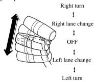
The direction indicators in the instrument cluster flash according to the operation of the direction indicator lever to show which signal is working.
