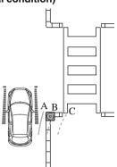
Make sure that there are no obstructions within the projected vehicle path lines. Turn the steering wheel so that the projected vehicle path lines travel inside of the obstruction (A), and drive the vehicle forward until it passes the obstruction. If the projected vehicle path lines are on an obstruction (B) or outside of the obstruction (C), the vehicle may contact the obstruction when turning the vehicle sharply.
