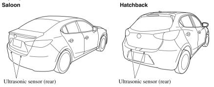
The ultrasonic sensors (rear) are mounted in the rear bumper.
