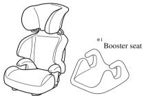
\*1 When using a booster seat, always install the vehicle head restraint to the seat where the booster seat is installed.
