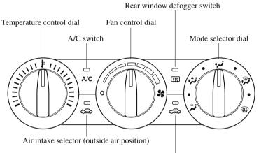
Air intake selector (recirculated air position)
