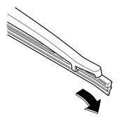
3. Remove the metal stiffeners from the blade rubber and install them in the new blade.
