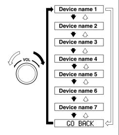
5. Press the audio control dial to select the device you would like to link.
