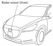
If the Smart Brake Support/Smart City Brake Support (SBS/SCBS) Warning Light (amber) is illuminated, the area around the radar sensor may be dirty. Refer to "Warning Guidance" in the centre display (Type B audio).
