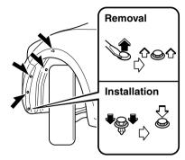
4. Turn the screw anticlockwise and remove it, and then partially peel back the mudguard.
