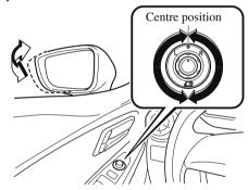
Type B To fold the mirrors, press the  $\rho$  mark on the outside mirror folding switch.
