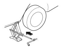
8. Turn the jack handle clockwise and raise the vehicle high enough so that the spare tyre can be installed. Before removing the wheel nuts, make sure your Mazda is firmly in position and that it cannot slip or move.
