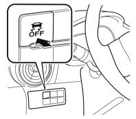
Press the switch again to turn the TCS/DSC back on. The DSC OFF indicator light will turn off.
