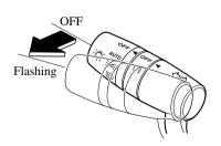
The headlight high-beam indicator light in the instrument cluster illuminates simultaneously. The lever will return to the normal position when released.
