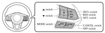
When the MODE switch is pressed, the MRCC main indication (white) turns on and the vehicle speed and the distance between vehicles while in headway control can be set.
