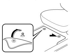
When setting a floor mat, position the floor mat so that its grommets or retainers are inserted over the pointed end of the retention posts.
