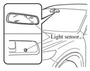
• The auto-dimming function is cancelled when the ignition is switched ON and the shift/selector lever is in reverse (R).
