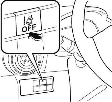
The Lane-keep Assist System (LAS) & Lane Departure Warning System (LDWS) OFF switch indicator light turns on.
