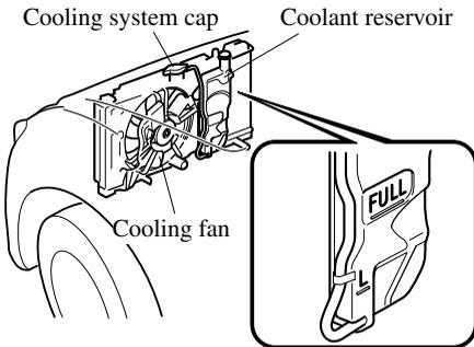
If it is at or near L, add enough coolant to the coolant reservoir to provide freezing and corrosion protection and to bring the level to F or FULL.
