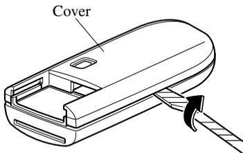
5. Remove the battery cap, then remove the battery.
