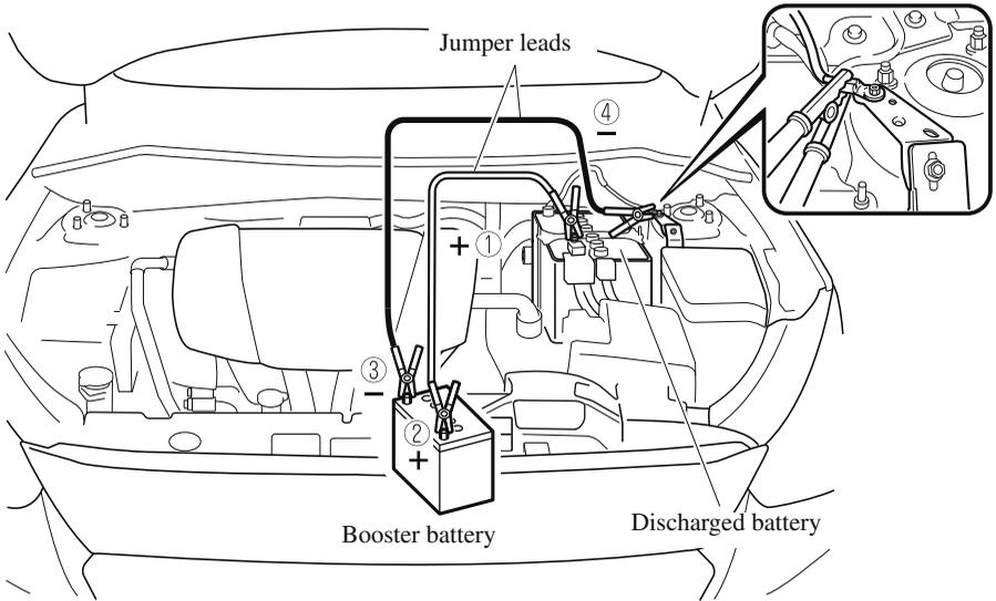
5. Start the booster vehicle's engine and rev the engine.
