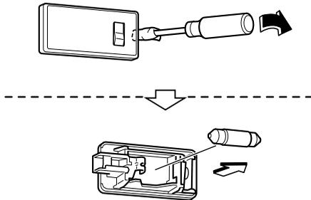
3. Install the new bulb in the reverse order of the removal procedure.
