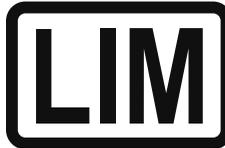
**▼ Speed Limiter Warning Beep****Indicated in instrument cluster**
