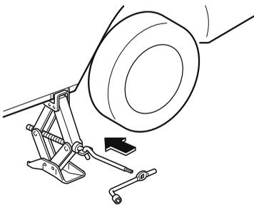
8. Turn the jack handle clockwise and raise the vehicle high enough so that the spare tyre can be installed. Before removing the wheel nuts, make sure your Mazda is firmly in position and that it cannot slip or move.
