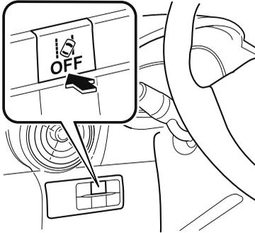
2. Drive the vehicle in the centre of the driving lane while the LDWS OFF indicator light is turned off. The system becomes operational when all of the following conditions are met.
