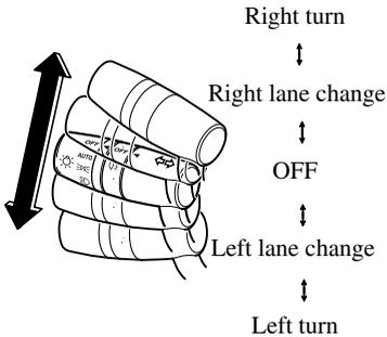
The direction indicators in the instrument cluster flash according to the operation of the direction indicator lever to show which signal is working.
