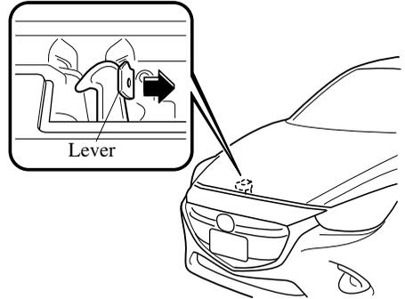
3. Grasp the support rod in the padded area and secure it in the support rod hole indicated by the arrow to hold the bonnet open.
