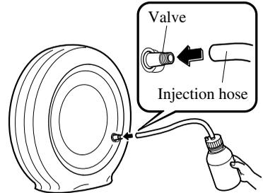
10. Hold the bottom of the bottle upright, squeeze the bottle with your hands, and inject the entire amount of tyre sealant into the tyre.
