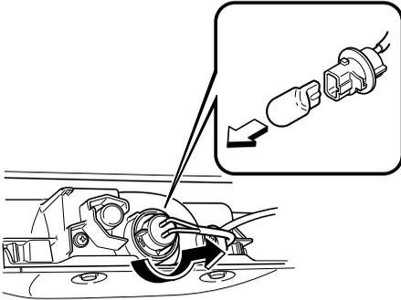
4. Install the new bulb in the reverse order of the removal procedure.
