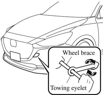
4. Hook the towing rope to the towing eyelet.
