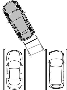
2. After the vehicle starts entering the parking space, stop and adjust the steering wheel so that the distance between the vehicle width lines and the sides of the parking space on the left and right are roughly equal, and then continue backing up slowly.
