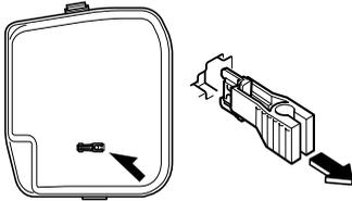
4. Inspect the fuse and replace it if it is blown.
