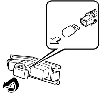
7. Install the new bulb in the reverse order of the removal procedure.
