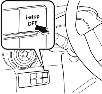
By pressing the switch until a beep sounds, the i-stop function is turned off and the i-stop warning light (amber) in the instrument cluster turns on. By pressing the switch again until the beep sounds, the i-stop function becomes operational and the i-stop warning light (amber) turns off.
