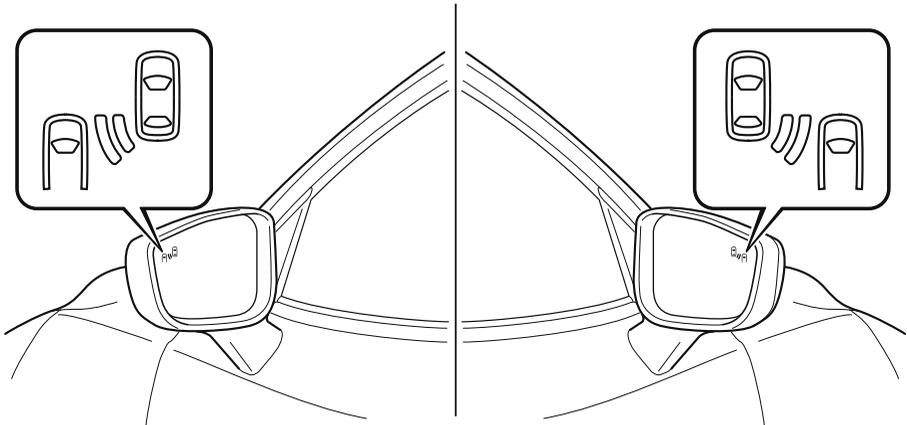
When the ignition is switched ON, the warning indicator light turns on momentarily and then turns off after a few seconds.
