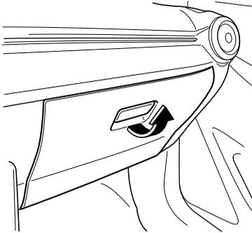
To close the glove compartment, firmly press in the centre of the glove compartment lid.
