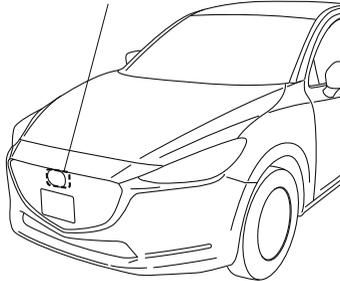
If the Smart Brake Support/Smart City Brake Support (SBS/SCBS) Warning Light (amber) is illuminated, the area around the radar sensor may be dirty. Refer to “Warning Guidance” in the centre display (Type B audio).
