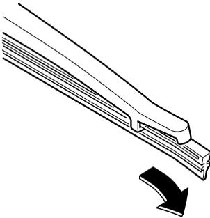
3. Remove the metal stiffeners from the blade rubber and install them in the new blade.
