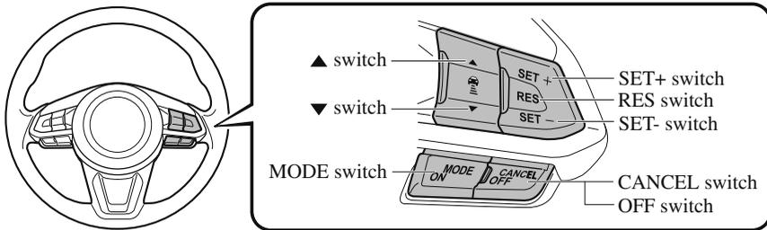
When the MODE switch is pressed, the MRCC main indication (white) turns on and the vehicle speed and the distance between vehicles while in headway control can be set.
