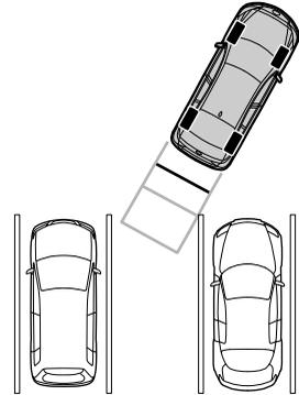
3. After your vehicle begins entering the parking space, continue backing up slowly so that the distance between the vehicle width lines and the sides of the parking space on the left and right are roughly equal.
