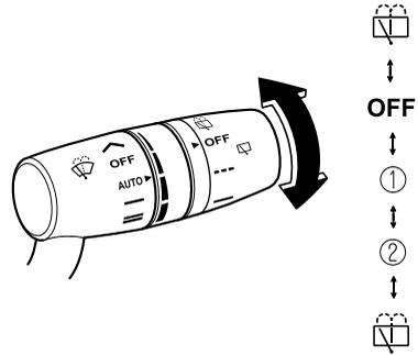
Turn the wiper on by turning the rear wiper/washer switch.
