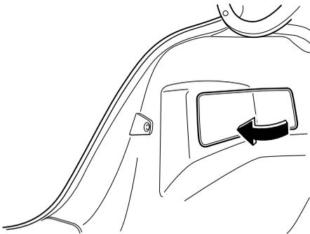
3. Turn the socket and bulb assembly anticlockwise and remove it.
