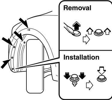
4. Turn the screw anticlockwise and remove it, and then partially peel back the mudguard.
