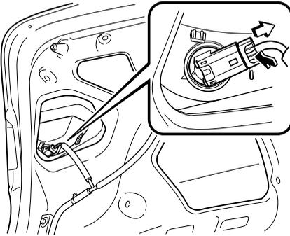
5. Turn the socket and bulb assembly anticlockwise and remove it.
