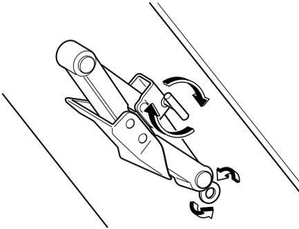
3. Turn the wing bolt completely to secure the jack.
