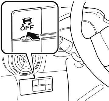
Press the switch again to turn the TCS/DSC back on. The DSC OFF indicator light will turn off.
