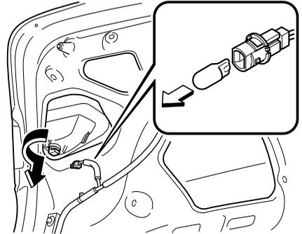
7. Install the new bulb in the reverse order of the removal procedure.
