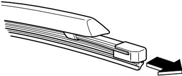
5. Remove the metal stiffeners from each blade rubber and install them in the new blade.
