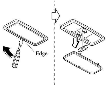
3. Install the new bulb in the reverse order of the removal procedure.
